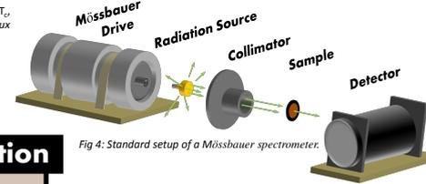
Fig 4: Standard setup of a Mössbauer spectrometer.
